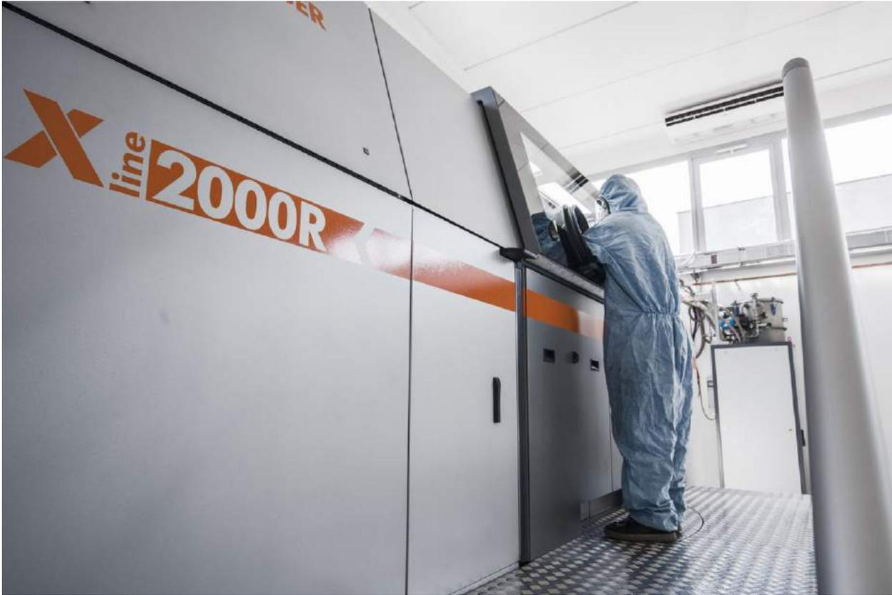
Fig. 11 A large format Concept Laser X Line 2000R PBF-LB machine (Courtesy BEAMIT)
